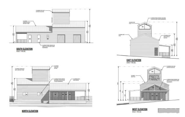
Figure 7: Elevations. Source: SEE and Plans
