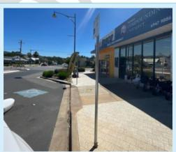
Implement shared areas with yellow diagonal linemarking for <u>all</u> 45-degree accessible on-street parking spaces in accordance with Section 4.5.2 of AS2890.5:2020.
